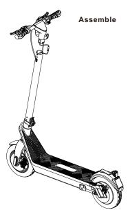
1. Unfold the pole and fasten the folding
