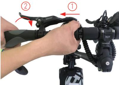
1、Expand the left handle method, hold the fixed joint slider with one hand, slide the slider to the far left and fix it.
