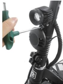
Adjust the position of headlight and horn, tighten the fixing bolts with a hexagon wrench. Attention, don't change the direction for horn, otherwise it will cause the horn bracket to break.
