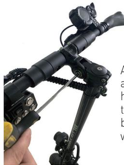
Adjust the position and height of the handlebar and tighten the fixing bolt with a hexagon wrench.
